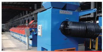
High speed straight line wire drawing machine. It can produce 1.5 mm to 5 mm.
